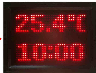
(8) Upper- Show Days of a week (abbr./) Date, Temperature, % of Humidity; it alternately shows each value and changes every 10 seconds. Lower- Show Time of Hour:Minute
