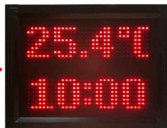
(9) Upper- Show % of Humidity, Temperature, Date and Month (numeric value); it alternately shows each value and changes every 10 seconds. Lower- Show Time of Hour:Minute
