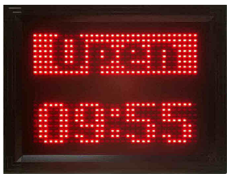
(TEST) Upper- Alternately Show flashing message" Open" and "Closes" by pressing this Key Lower- Show Time of Hour:Minute
