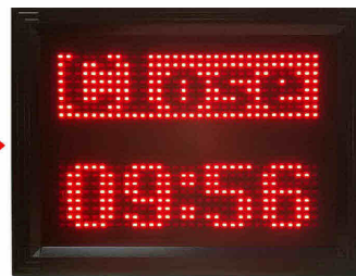
(TEST) Upper- Alternately Show flashing message" Open" and "Closes" by pressing this Key Lower- Show Time of Hour:Minute
