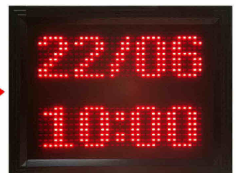
(9) Upper- Show % of Humidity, Temperature, Date and Month (numeric value); it alternately shows each value and changes every 10 seconds. Lower- Show Time of Hour:Minute
