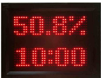
(9) Upper- Show % of Humidity, Temperature, Date and Month (numeric value); it alternately shows each value and changes every 10 seconds. Lower- Show Time of Hour:Minute
