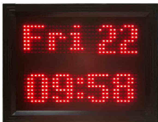
(8) Upper- Show Days of a week (abbr./) Date, Temperature, % of Humidity; it alternately shows each value and changes every 10 seconds. Lower- Show Time of Hour:Minute
